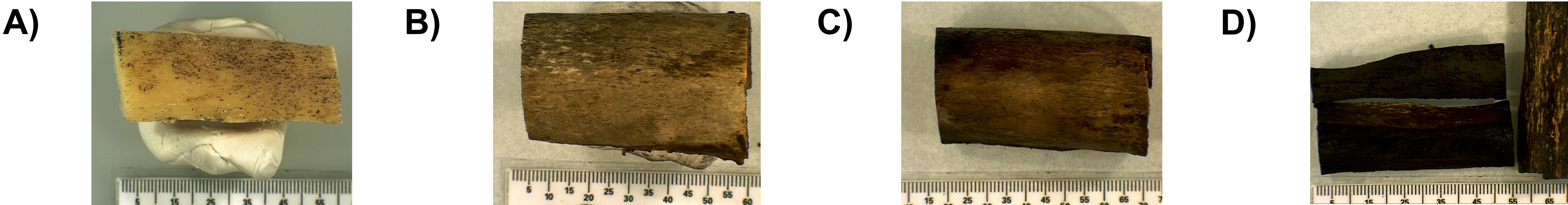
Figure 1. Representative Photos of Femur Cross-sections Thermally Degraded to Different Stages Based on Bone Color. One window cut was reserved as an A) Unburned control. The remaining cross-sections were thermally degraded to B) Burned, Light Brown; C) Burned, Brown; and D) Burned, Black color stages.
